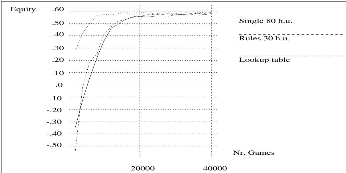
Figure 4.6: The results obtained by the lookup tables compared to the large single network and the architecture which uses symbolic rules to select an expert network. The use of lookup tables results in faster learning and a better final performance.
